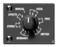
The **Presets** for the Blue Max are controlled by this sixteen position rotary encoder. As the encoder is rotated, parameters are digitally switched, simultaneously controlling attack, release, ratio and threshold.
