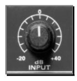
The **Input** control adjusts the gain on the input amplifiers for both channels. Amplification gain varies widely from -20dB to +40dB. The large range is necessary to amplify instruments such as guitar. Thus the input stage to the Blue Max is actually a pre-amp.
