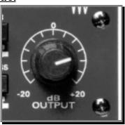
The Output control is used to set the desired output of the Blue Max. It is sometimes referred to as 'gain makeup' control. This terms is derived from the fact that as the compressor lowers the output level during gain reduction, the overall signal level is lowered, requiring the user to 'makeup' the gain thereby restoring the original signal level.
