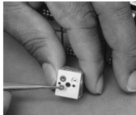
Figure 5.10: DH200 Transducer O-Ring Replacement
