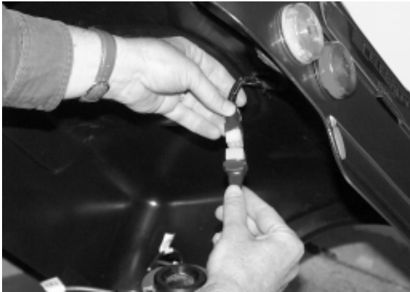
Figure 19. Disconnecting The Lighting Harness
