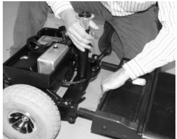
Figure 26. Separating The Frame
