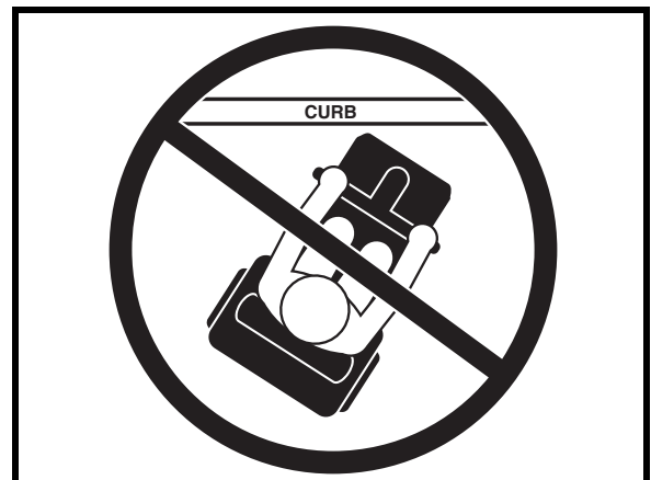
Figure 3A. Incorrect Curb Approach
