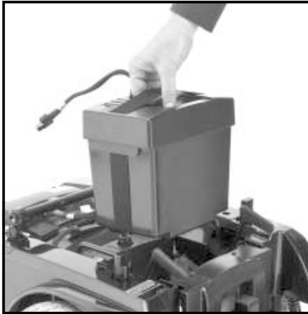
Figure 16. Removing Battery Boxes
