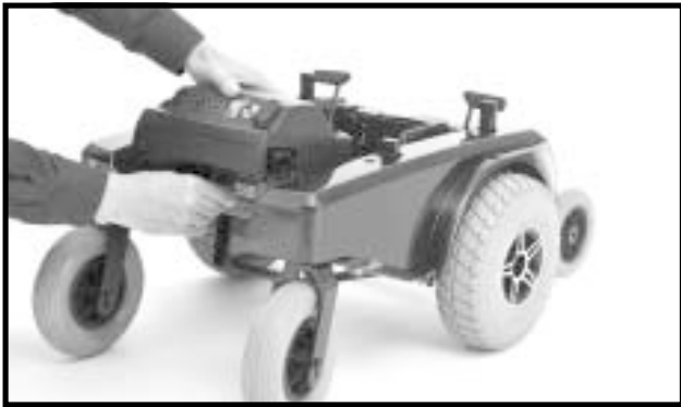
Figure 17. Removing Battery Well Frame
