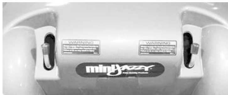
Figure 5. Freewheel Mode (Drive Motor Disengaged)
