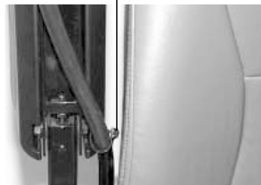
Figure 11. Wire Tie Location
