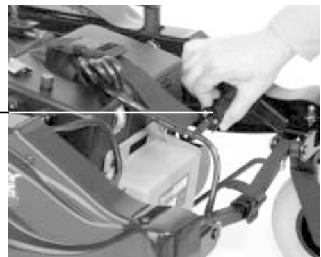
Figure 16. Disconnecting the Motor Harness Connector
