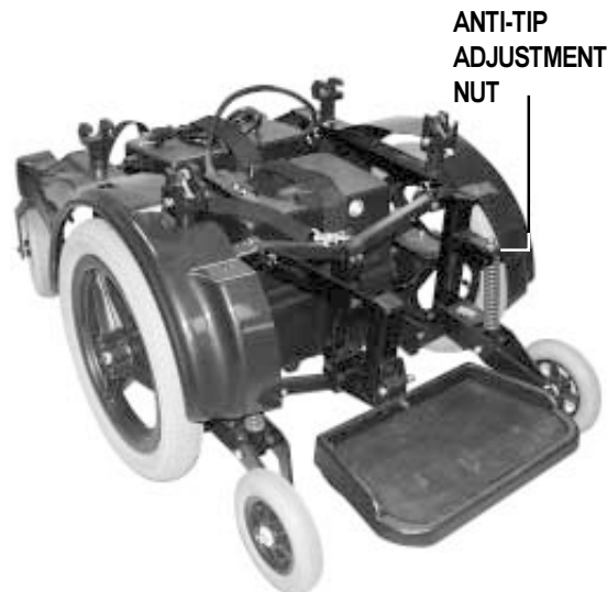
Figure 13. Anti-tip Wheel Adjustment
