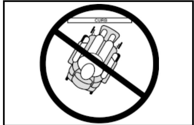
Figure 3. Incorrect Curb Approach
