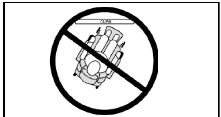
Figure 3. Incorrect Curb Approach
