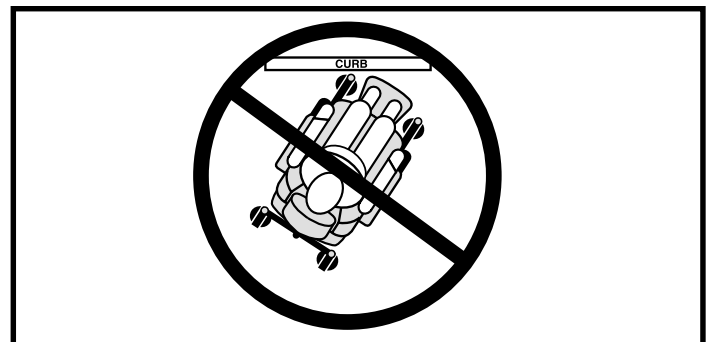
Figure 3. Incorrect Curb Approach
