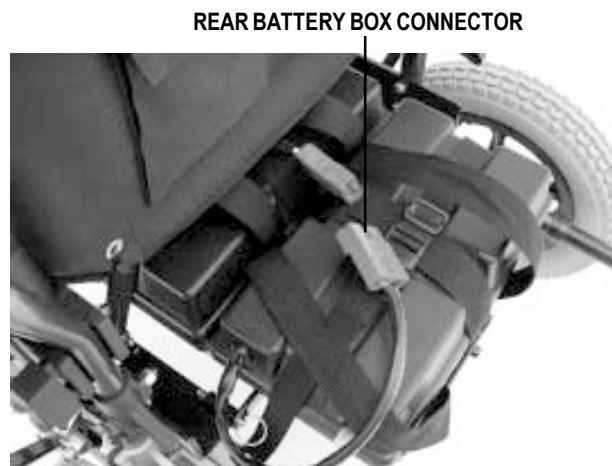
Figure 16. Rear Battery Box
