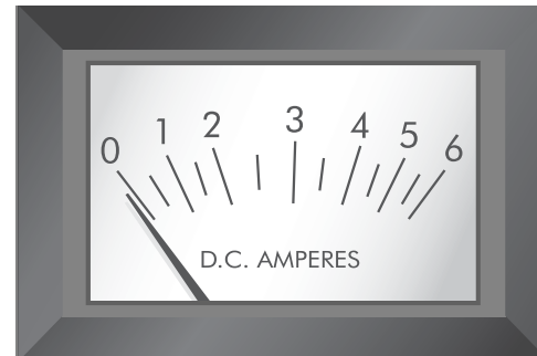
FIGURE 10. AMMETER INDICATES BATTERY IS FULLY CHARGED
