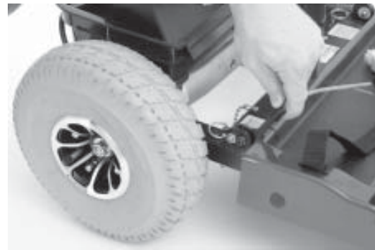
FIGURE 24. LIFT UP FRAME LOCK LEVER TO UNLOCK
