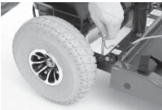
FIGURE 23. REMOVE BALL DETENT PINS
