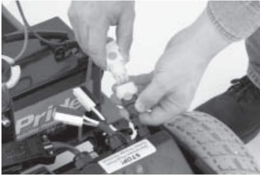
FIGURE 19. DISCONNECTING THE FRONT-TO-REAR HARNESS
