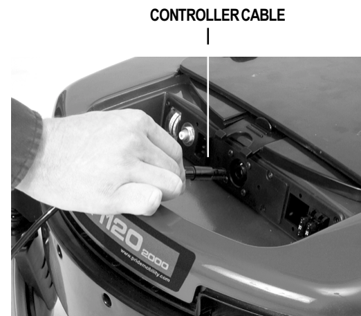
Figure 11. Controller Cable Connection
