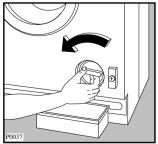
Unscrew and remove the filter.
