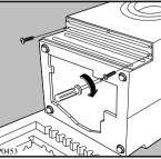
Set the machine upright and remove the two remaining bolts from the back.
