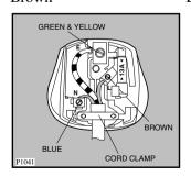
The wire coloured green and yellow must be connected to the terminal marked with the letter  $\ll E \gg$  or by the earth symbol  $\frac{1}{=}$  or coloured green and yellow.
