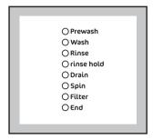
The pilot lights corresponding to the different phases making up the selected programme light on.
