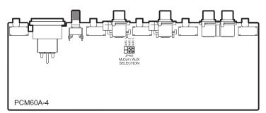
NOTE: The unit provides a Phantom Power DC 15V for electric condenser microphone, unit comes with jumper set to Phantom Power enable ON.
