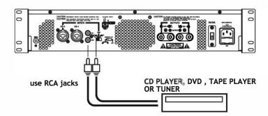
Connecting an equalizer or external signal processor Connect the processor's OUT to the amplifier's INPUT connectors.
