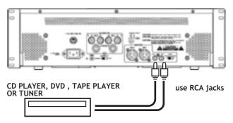
**Connecting an equalizer or external signal processor** Connect the processor's OUT to the amplifier's INPUT connectors.
