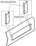
4. Open the two pieces of rubber cover on the unit to display the four screw holes, and then use four screws (M4X30) to mount the unit to the dashboard with the mounting plate between the dashboard and the unit.
