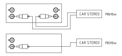
CAR SIGNAL INPUT (RCA LINE OUT) MUST BE CONNECTED TO ONLY EACH "L" CHANNEL (BRIDG SWITCH KNOB SHOULD BE SELECTED MO). IF CAR SIGNAL INPUT IS CONNECTED TO "R" CHANNEL THERE SHALL BE NO POWER OUT (NO SOUND).
