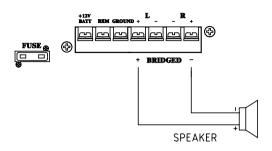
SPEAKERS NEGATIVE TERMINALS ON AMPLIFIER ARE NOT USED IN BRIDGED MODE BRIDGING IS DONE BY SUMMING POSITIVES.
