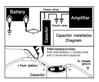
**Note**: Capacitors are most effective when there is a 18" (0.5m) or less of wire between the cap and the amplifier(s).
