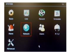
Put a checkmark in the box after Obtain an IP address automatically. Click TEST button, if you get OK message at the bottom. Click Apply and Exit.
