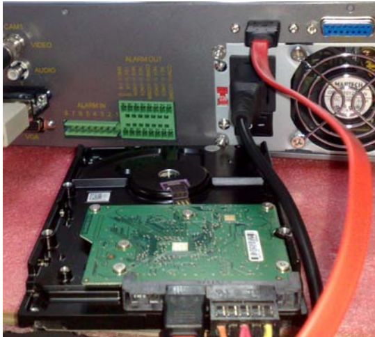
Fig. B-2 Normal Hard Drive Connection
