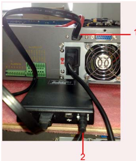
Fig. A-1 Portable Hard Drive Connection
