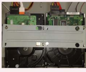
Fig 2.1 Installing hard drive
