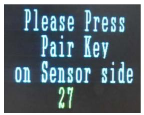
Press the Pair the button on corresponding camera and wait for a while, the monitor connected to the receiver will display the images from the cameras that have been matched. Pairing succeeded.
