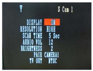
Through **Right/Left** button can adjust parameters, and through **Up/Down** button can select the features to set.
