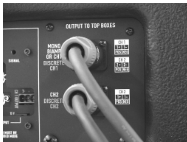
Speakons provide a clean appearance, reliable electrical connection and positive locking mechanism. To remove a Speakon, pull the thumb-latch back and twist counterclockwise 1/8th turn.
