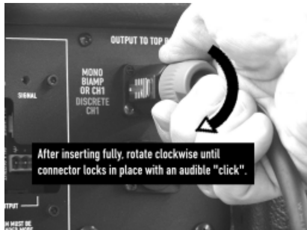
When the Speakon locks into place, an audible "click" confirms connection.
