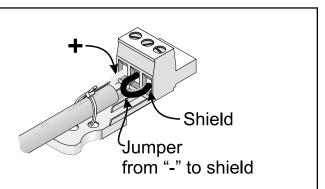
**Unbalanced inputs can be used if required.** If unbalanced audio sources are used, it is preferable to use an appropriate audio transformer (or other unbalanced-to-balanced "converter") to provide a balanced input to the DSP-3. If this is not possible, then it is recommended that the negative terminal and shield terminal be connected to one another with a jumper wire.
