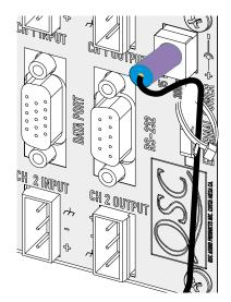
Insert the coaxial power plug into the EXTERNAL POWER jack. Ensure that the plug is firmly seated in the jack. Use the "tab" provided on the chassis for securing the power cord with a tie-wrap (wire-tie).
