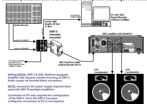
DSP-3 Remotely Mounted used with QSC DataPort Amplifier. Audio Input via Terminal Block Inputs
