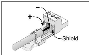
**Balanced connection is recommended for all inputs.** The terminal block inputs on the DSP-3 are electronically balanced. Balanced input cables are recommended to minimize noise pick up and prevent ground loops.
