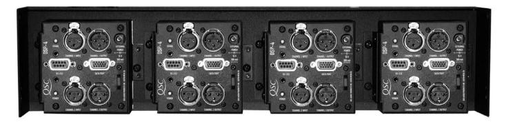
A remote rack mounting bracket (the DPX-4) is available to use with PowerLight, 4-channel QSC amplifiers, or for non DataPort equipped amplifiers. Designed to be bolted to the rear of an amplifier rack, up to four modules can be mounted to each panel, providing up to **eight** channels of DSP processing in a three rack unit space.
