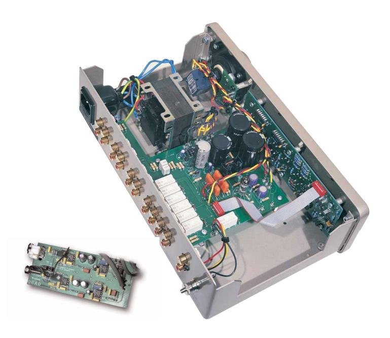
A completely new design, the QC-twenty-four pre amplifier is both neutral and detailed. Using a military specification 6111 valve, which is so reliable, it's hardwired to the circuit board.
