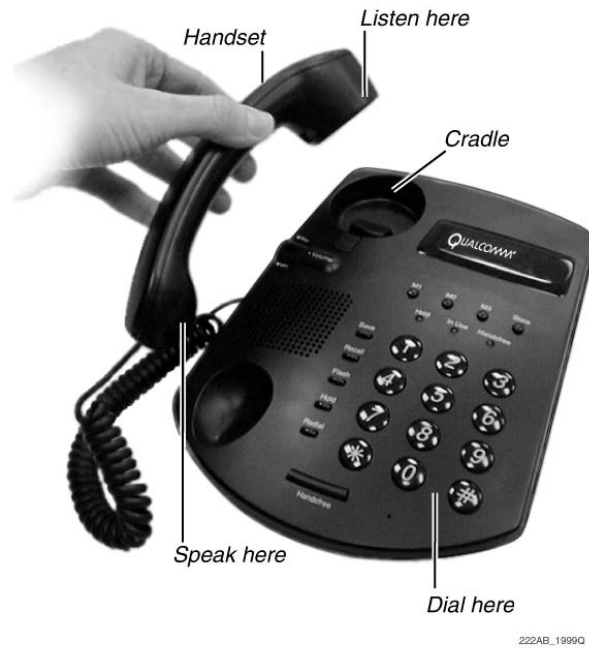
Figure 1. Telephone showing relevant user features
