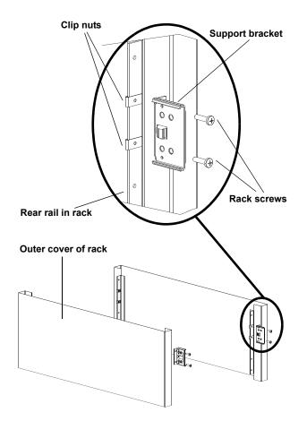
**4** With the help of a second installer, insert the autoloader into the rack so that the autoloader brackets slide into corresponding support brackets on the rear rails and the tabs at the front of the autoloader align flush with the clip nuts on the front rails (see <u>figure 5</u>).
