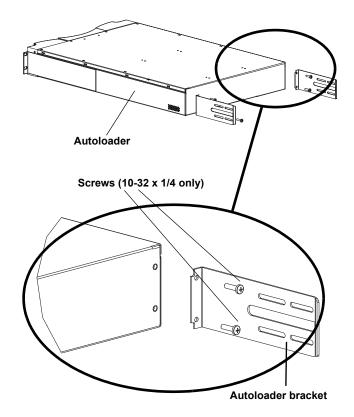
**3** Using rack screws, attach a support bracket to the clip nuts on each rear rail (see <u>figure 4</u>.)
