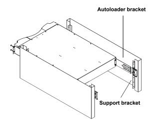
5 While the other installer holds the front end of the autoloader, secure the front end of the autoloader to the rack using four rack screws (two per tab) as shown in <u>figure 6</u>. Tighten the screws just enough to secure the autoloader to the front rails.
