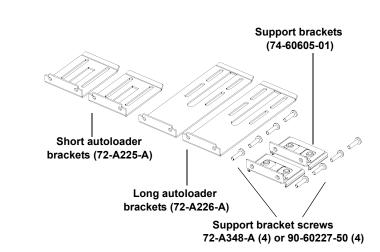
Figure 1 Rack Mount Hardware
