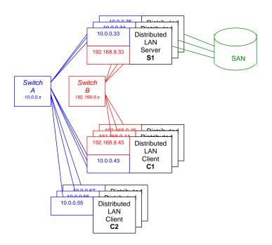
In the diagram there are two subnetworks: the blue subnetwork (10.0.0.x) and the red subnetwork (192.168.9.x). Servers such as S1 are connected to both the blue and red subnetworks, and can each provide up to
