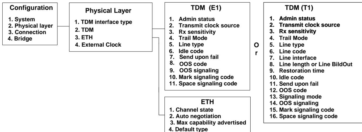
Figure 3-3. Configuration > Physical Layer > TDM and ETH Configuration
