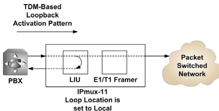
Figure 6-14. T1 Inband Loopback Performed by Local IPmux-11
