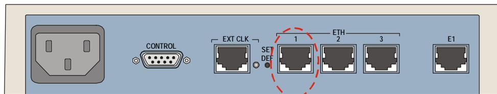
Figure 2-2. ETH 1 Electrical Connector
