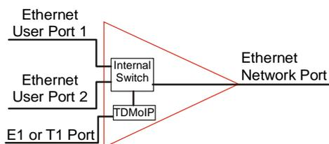
Figure 1-11. IPmux-11 with Two Ethernet User Port
