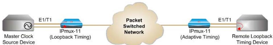
Figure 1-5. IPmux-11 in Adaptive Timing Mode
