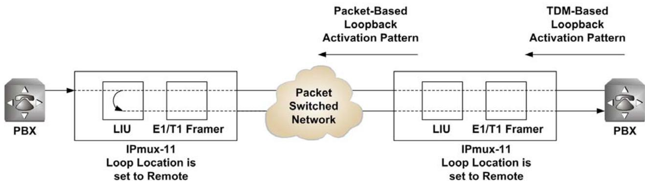
Figure 6-15. T1 Inband Loopback Performed by Remote IPmux-11
