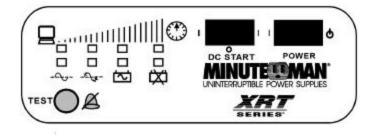
XRT600 Front Panel Showing Load LED's
