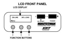
The XRT1000 through XRT2000 units have a 32 character LCD display, three push buttons, and the Pow er On and DC Start switches. (Both 120 and 220 VAC versions)
