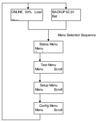
The Mode Display will be shown after the unit's first power up diagnostics have been run, or when it is selected by stepping through the menu selections.
