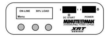
If an alarm condition exists, the condition will be reported on the front panel. If no AC Pow er is present and the battery is charged, pressing the DC START switch for approximately 5 seconds will bring up the UPS in the inverter mode and provide pow er to the protected equipment from the battery.
