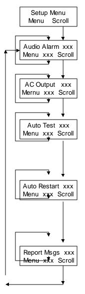
**Note:** At any step in the "Setup" menu, pressing the "MENU" selection will move you to the "Config" menu.
