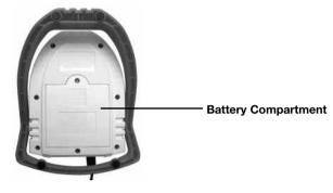
On the back of the main unit, loosen the screw on the battery compartment and insert four (4) "AA" batteries as indicated inside the compartment (alkaline batteries recommended). Replace the battery compartment door.
