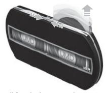
1. Eject UMD's by sliding the button as shown
