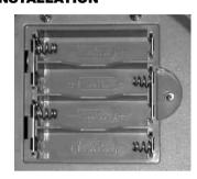
On the back of the main unit, loosen the screw on the battery compartment and insert four (4) "AA" batteries as indicated inside the compartment (alkaline batteries recommended). Replace the battery compartment door.
