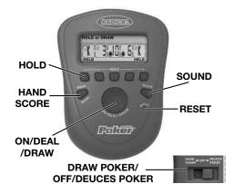
SOUND button - Press to turn the sound on/off.
