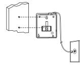
supplied) into each hole, letting the heads extend about <sup>3</sup>/<sub>16</sub> inch (5 mm) from the wall. Connect the supplied long modular cord to the phone's line jack. Fit the keyhole slots over the screw heads and slide the phone downward to secure it. Plug the line cord into the telephone line jack.
