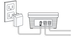
**Caution**: You must use a Class II power source that supplies 9 volts AC and delivers at least 400 mA. Its center tip must be set to positive and its plug must fit the TAD's **AC 9V** jack. The supplied adapter meets these specifications. Using an adapter that does not meet these specifications could damage athetoid or the adapter.
