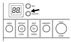
To erase all messages, while playback is stopped, hold down **DELETE**. The TAD sounds a long beep and **00** appears on the display.
