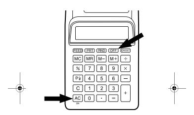
Press **AC** to turn on the EC-3031. Press **OFF** to turn it off.
