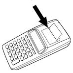
Replace the paper roll when you see a red strip on one edge of the paper. Use a standard  $2^{1/4}$ -inch paper roll, such as Cat. No. 65-710 or 65-715.
