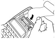
To use the external roll holder, insert the end of the paper into the rear slot from the bottom of the calculator. Then insert the end of the paper into the slot inside the compartment.
