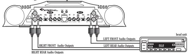
2 CHinput connections using low level inputs
