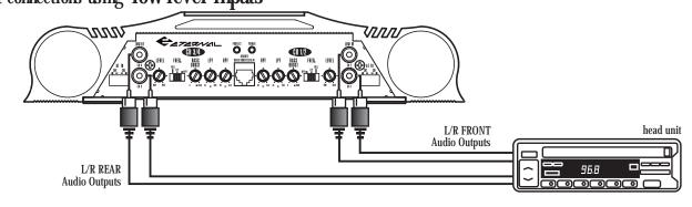
2 CHinput connections using low level inputs
