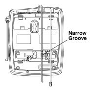
Plug the modular cord's other end into the wall plate jack, then align the bracket's keyhole slots with the wall plate studs and slide the base downward to secure it.
