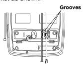
6. Align the bracket's keyhole slots with the mounting screws and slide the base downward to secure it.
