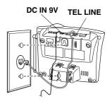
For a wall plate, plug the modular cord's other end into the wall plate jack, then align the base's keyhole slots with the wall plate studs and slide the base downward to secure it.
