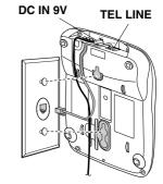
4. For a wall plate, plug the modular cord's other end into the wall plate jack, then align the base's keyhole slots with the wall plate studs and slide the base downward to secure it.
