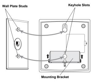
To mount the phone directly on a wall, in addition to the preceding steps, you need two screws (not supplied) with heads that fit into the keyhole slot on the bottom of the base.
