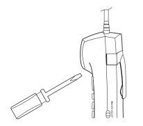
To replace the belt clip, insert either tab of the belt clip into one of the handset's slots, then snap the other tab into handset's other slot.
