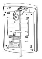
Insert the tabs on the narrow end of the bracket into the slots on the bottom of the base as shown and route the other end of the short modular cord through the center of the bracket. 4. Push the tabs on the wide end of the bracket into the lower slots on the bottom of the base.
