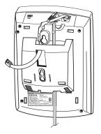
5. Plug the short modular cord's other end into the wall plate jack, align the base's keyhole slots with the wall plate studs, and slide the base downward to secure it.
