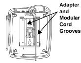
Plug the modular cord's other end into the wall plate jack, then align the bracket's keyhole slots with the wall plate studs and slide the base downward to secure it.
