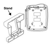
Insert the two tabs at the top of the narrow end of the supplied bracket into the base's upper tab slots as shown, then press down on the bracket's latches and insert them into the lower slots.
