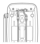
4. Plug the modular cord's other end into the wall plate jack, then align the base's keyhole slots with the wall plate studs and slide the base downward to secure it.
