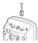
Insert the supplied AC adapter's barrel plug into the DC IN 9V jack on the back of the base.
