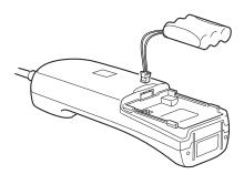
Plug the battery pack's connector into the socket in the compartment, (the connector fits only one way), replace the battery pack, and replace the cover.
